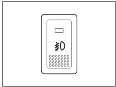
The front fog light comes on when the fog light switch is pushed in with the headlights
